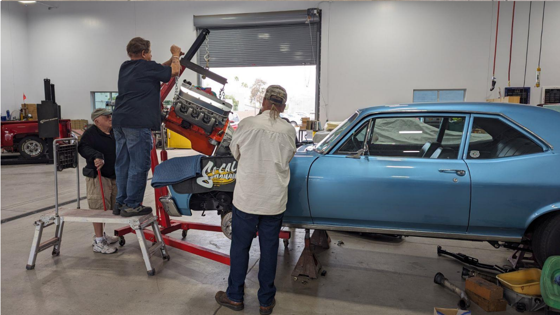
Len Manning installing his 454 Chevrolet with 540 hp on the Dyno. Photos Courtesy of Matthew Staske.
