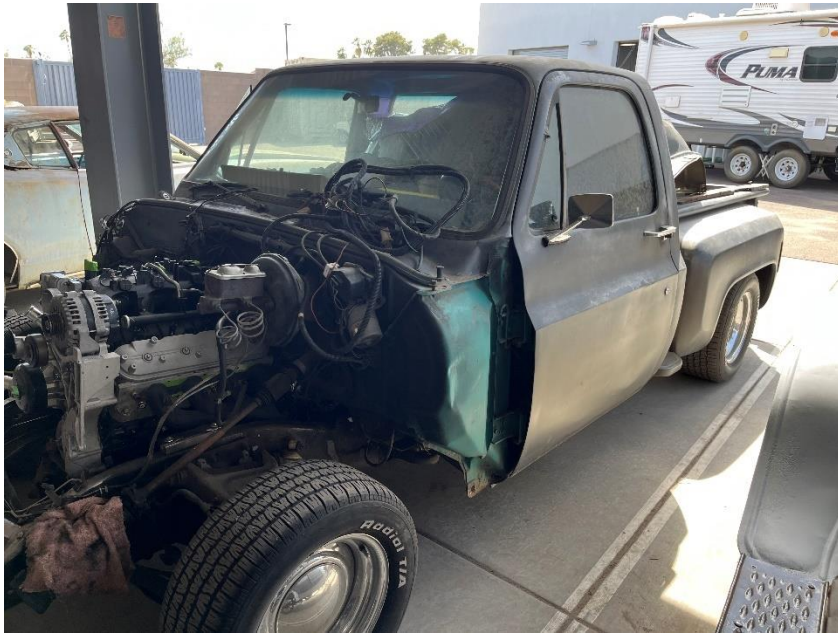
Stacy Benson is working on a 1973 Chev C-10 stepside. It has a 2004 Chev LS Engine paired with a Chev 4L80E automatic transmission.
